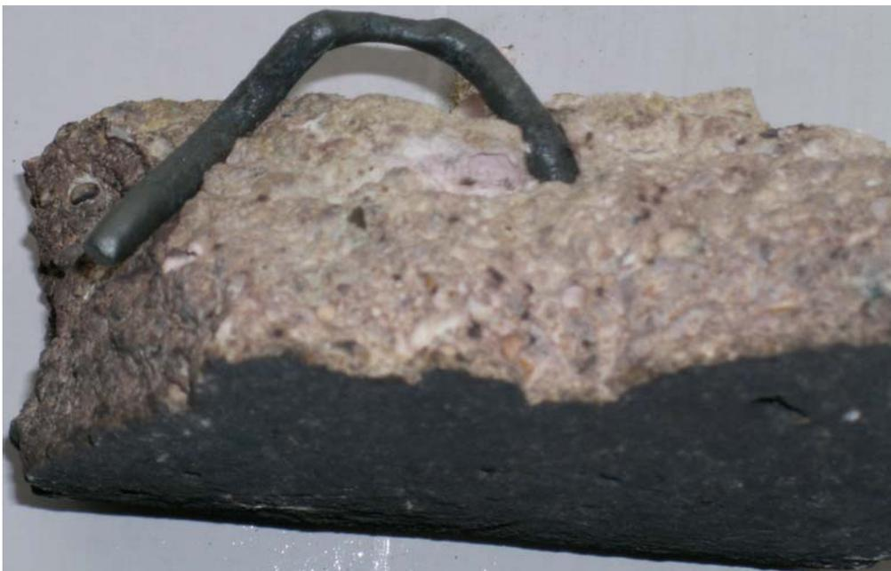
**Figure 1: Refractory with anchor showing partial weld fusion**
