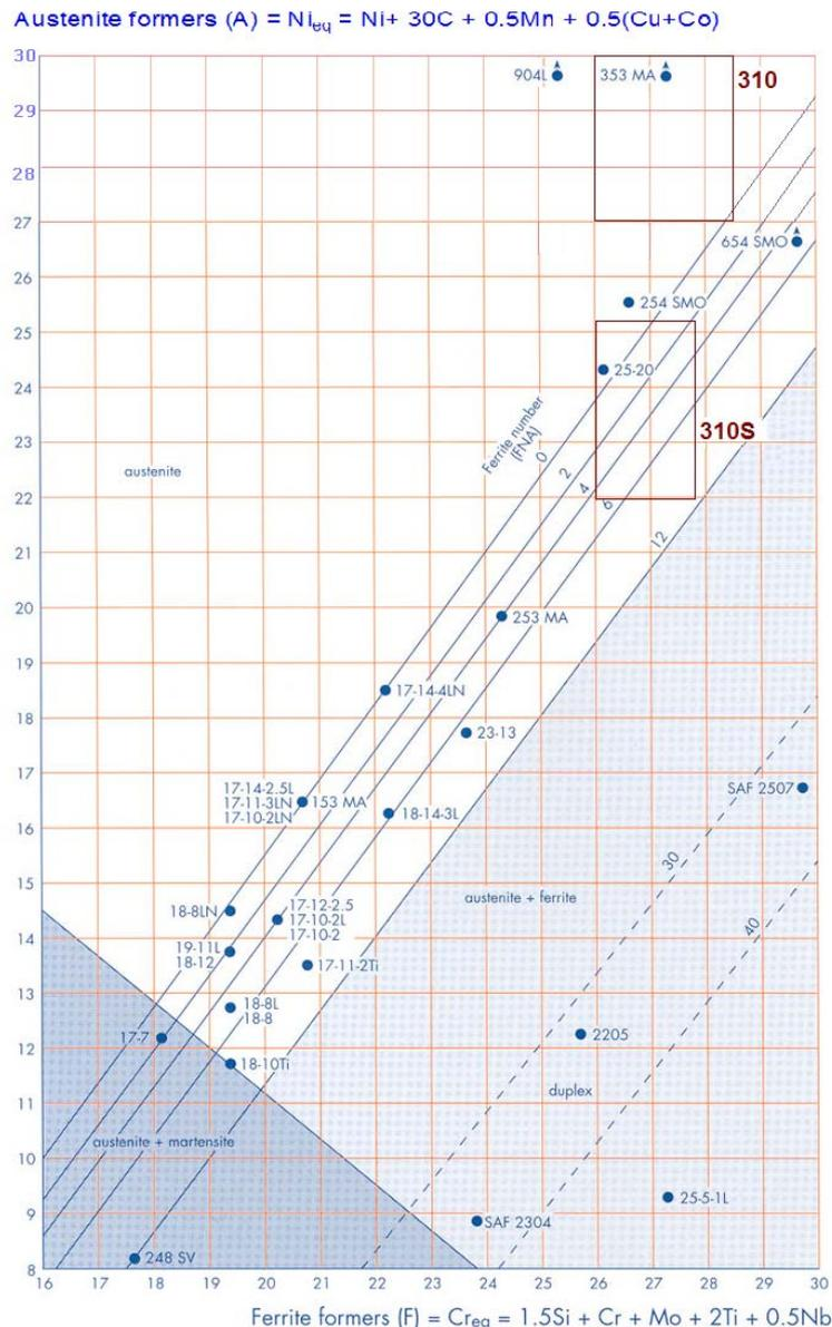
**Figure 5: Schaeffler-De Long Diagram**
