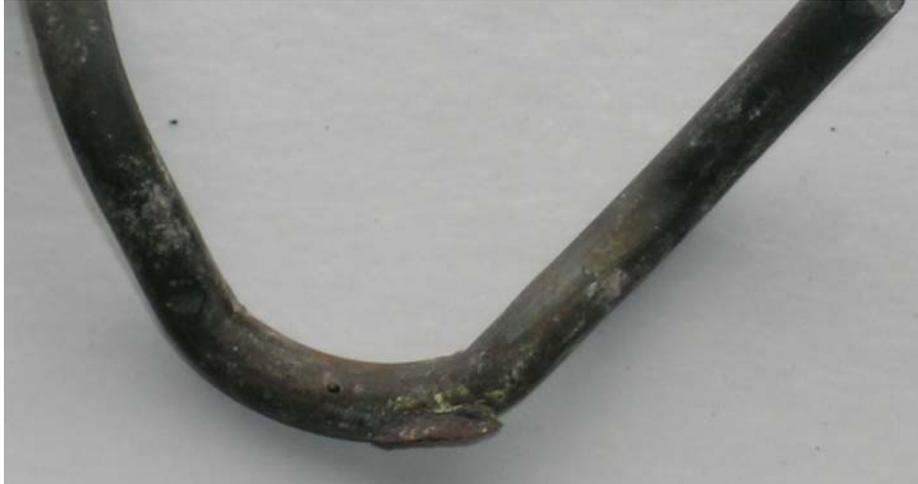
**Figure 2: V anchor with tack weld only taken from a “failed” castable system**
