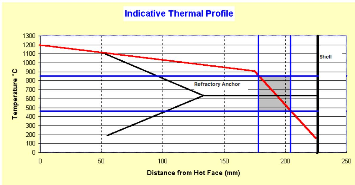
**Figure 4: Thermal profile through typical lining, highlighting the critical zone for  $\sigma$ -phase formation.**
