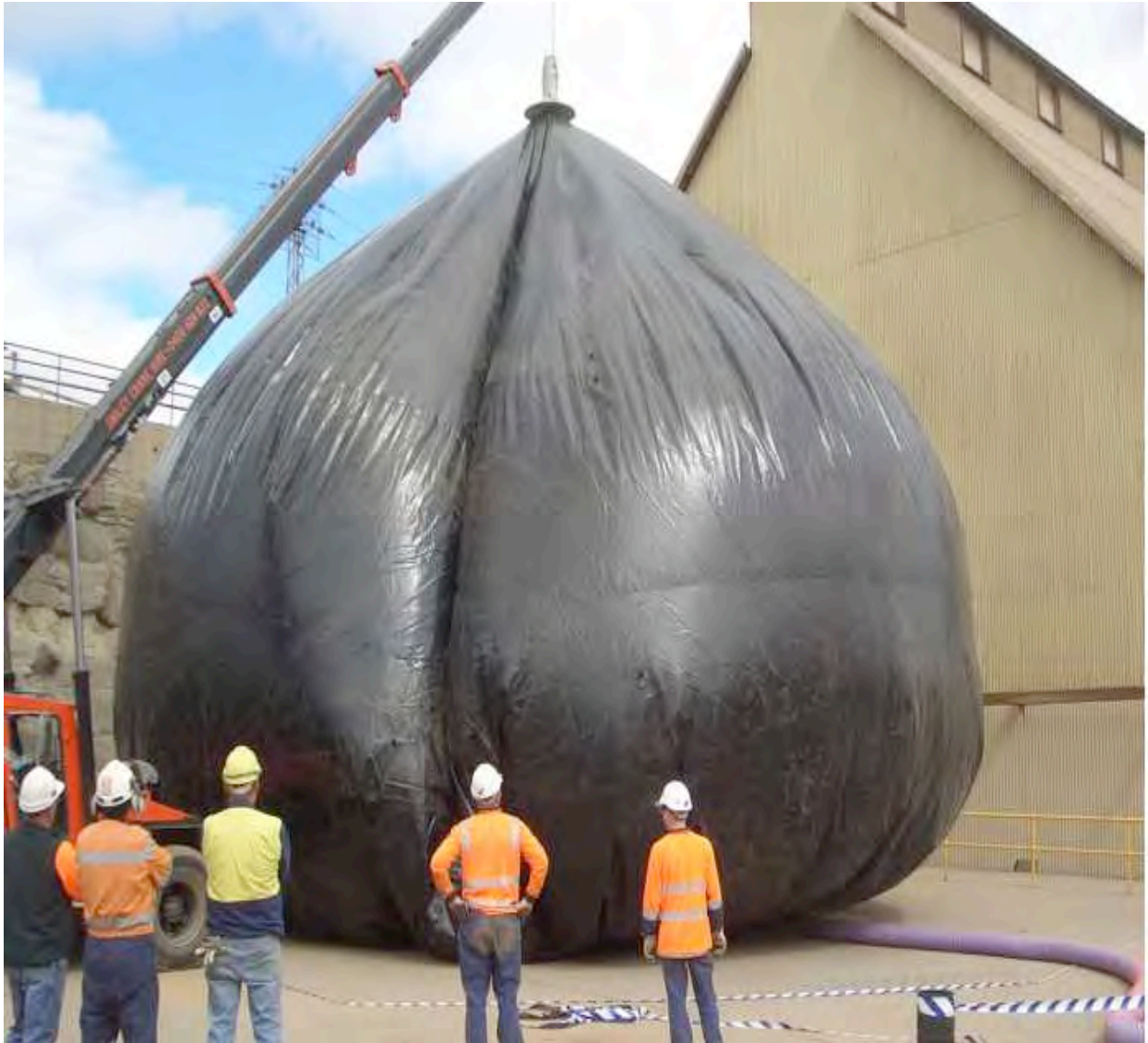
Figure 2: Large OPS undergoing inflation trials at factory in W. A.
